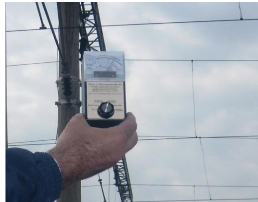
Fig. 5 Magnetometer under 27000V network; B = 7 mGs
