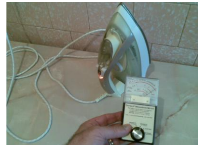
Fig. 2 Magnetometer near an energized iron; B=5 mGs
