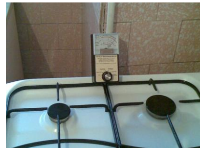
Fig. 1 Magnetometer near a gas pipe of a stove; B=5 mGs
