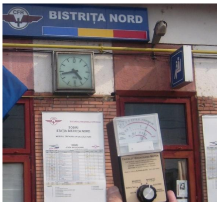
Fig. 4 Magnetometer at a height of 1.5 m; B = 6 mGs
